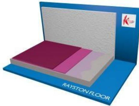
BASE: Concrete >28 days cured, moisture <4%, no capillary moisture, strength >1.5N/mm<sup>2</sup>, Temp. > 10°C, no contamination, grease, dust or open pores
