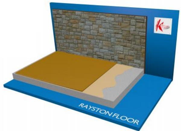
**ESPESOR APROXIMADO DEL SISTEMA: 30-40 mm**
