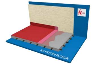
BASE: Concrete, >28 days curing, humidity <4%, no capillary moisture, strength <1.5N/mm2, Temp. > 10°C, without any type of contamination, grease, dust or open pore.
