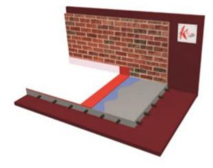
BASE: Concrete, >28-day curing time, humidity <4%, no rising damp, strength <1.5N/mm2, Temp. > 10°C, without any contamination, grease, dust or open pores.
